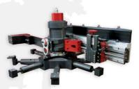
6 continuous groove facing feeds for a gramophone finish (ASME Standard) 3 different sized quick set independent bases for improved on-site operation Hardened slide ways to maintain long term accuracy Toolpost aids RTJ groove creation
