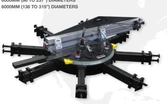
Precision flatness tolerances across large diameters Hydraulic high-torque anti-backlash drive Precision preloaded linear rotary drive Adjustable fast-set hydraulic chuck Rigid and adjustable mounting base Adjustable fast-set clamping jaws
